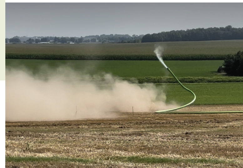
Manure hose rupture when the line is charged with pressurized air during line cleanout.
